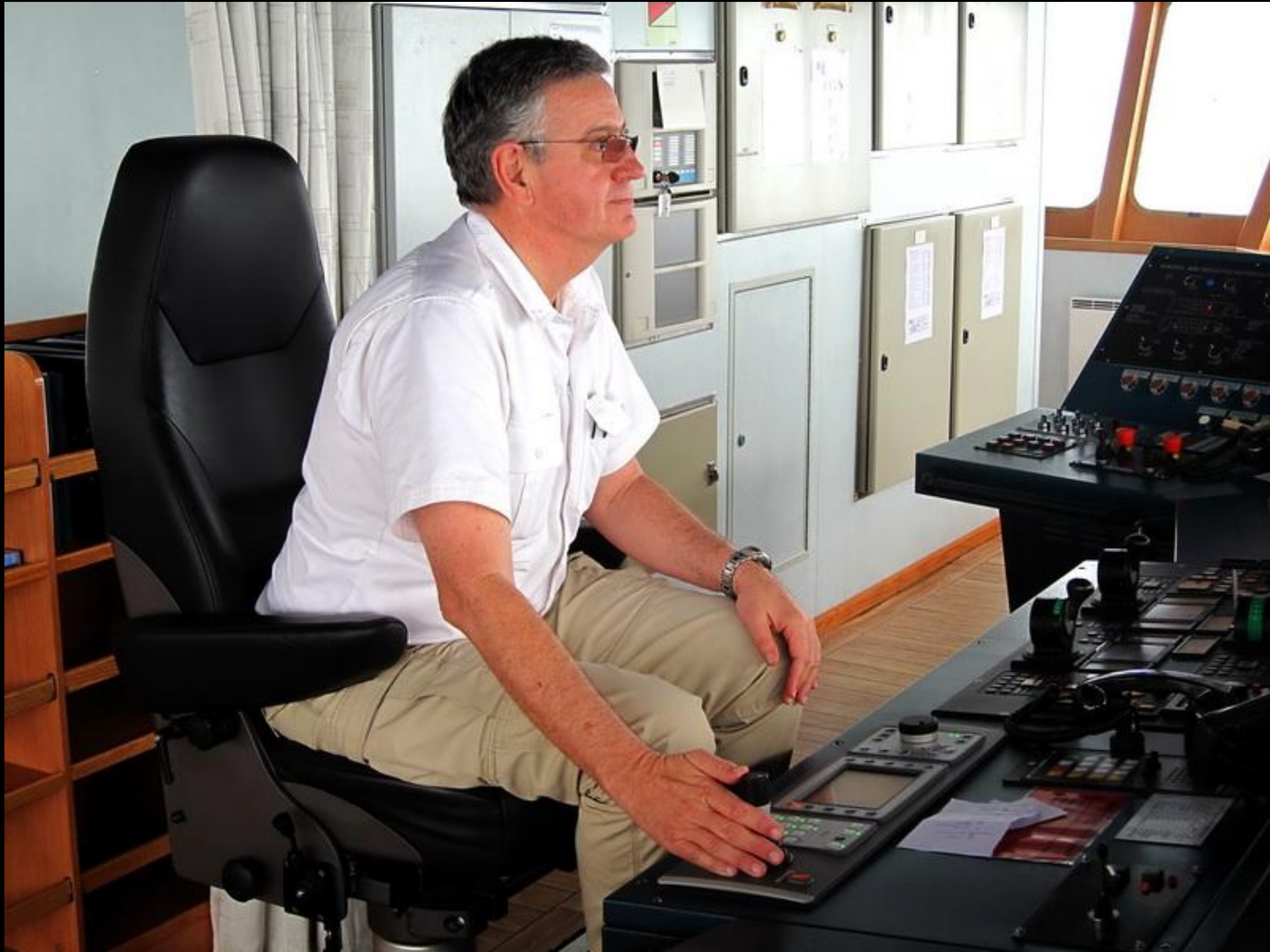
Capt. Daley is at the forward helm. The device in his hand is the joystick used for the DP-2 systems.
