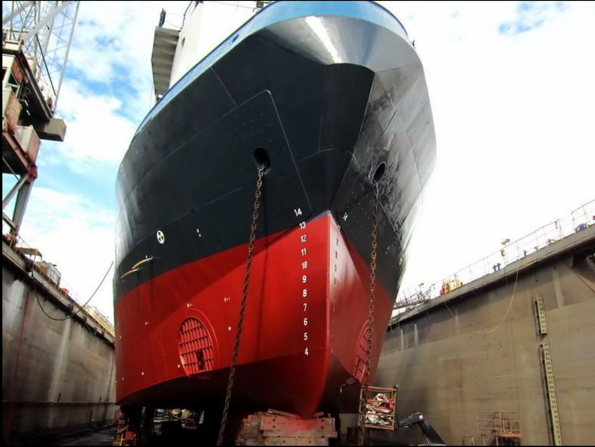
Voilà! The final coat of paint is applied.
