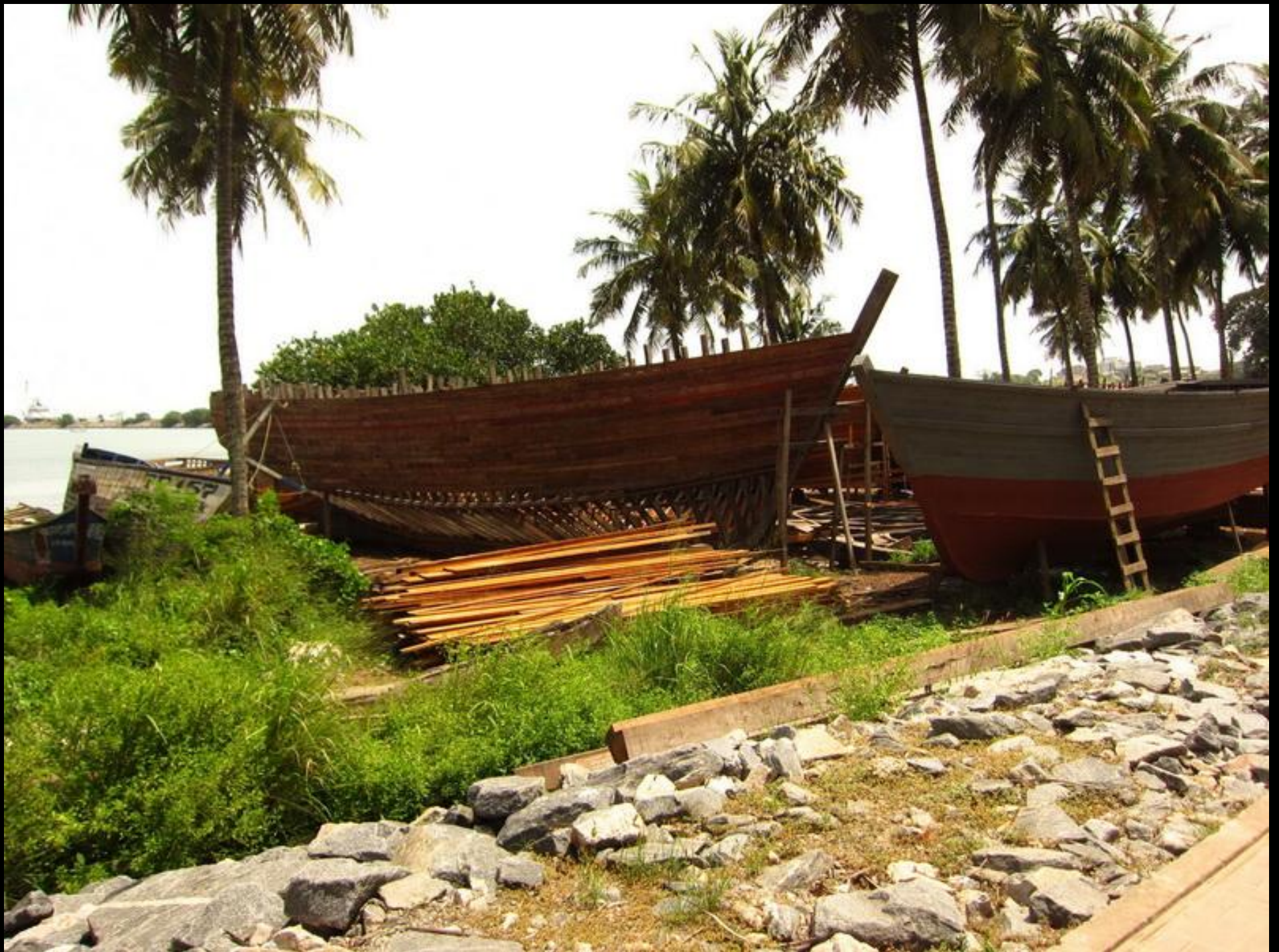
This mammoth fishing vessel is being built of mahogany laid one plank at a time by hand. What a beauty she will be when completed and should last a lifetime.
