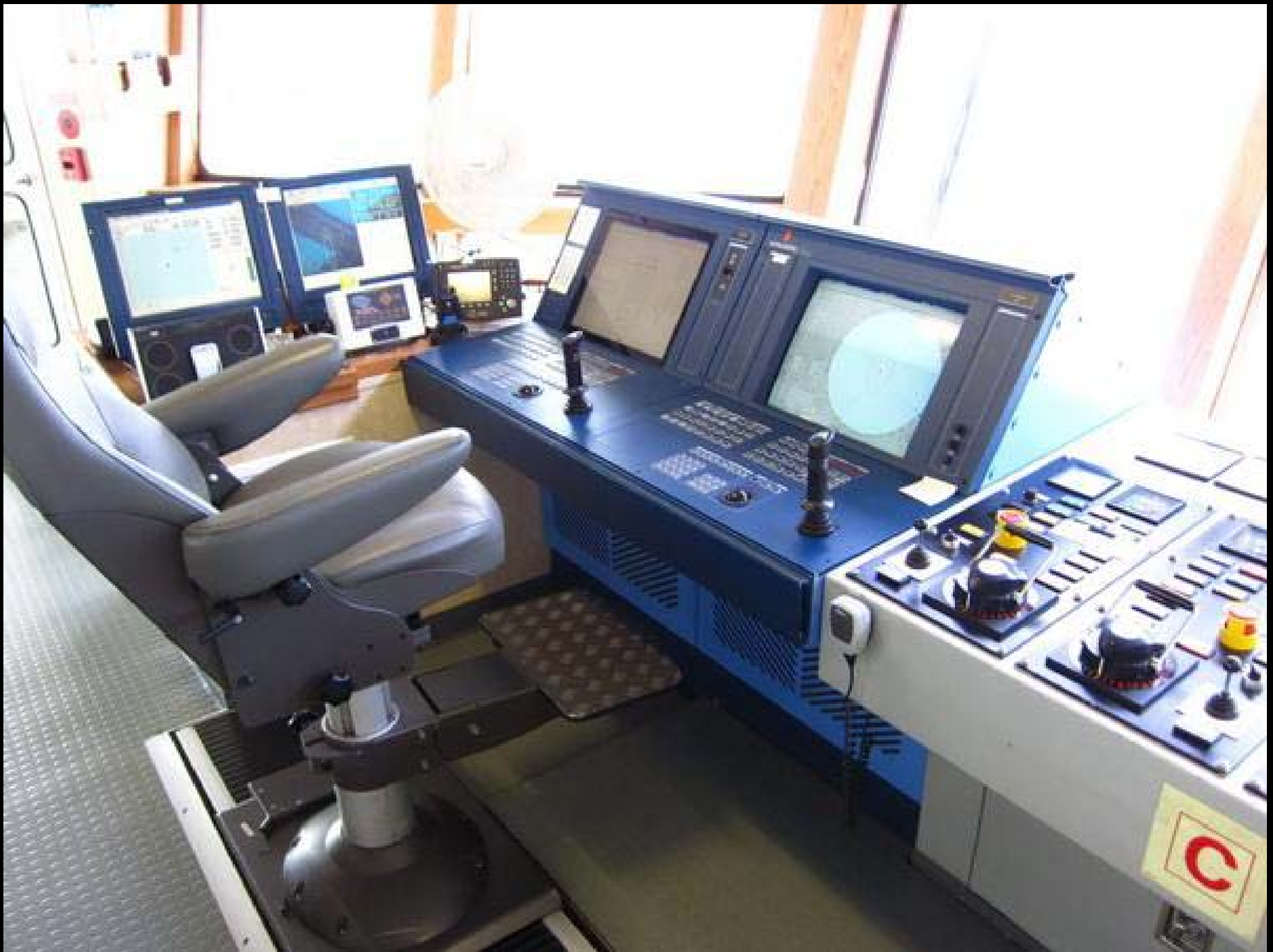
Screen to the left is the GPS. Next one to the right is the fan beam. Then there are two DP consoles. Two consoles and two computers are required to be a DP 2 vessel.
