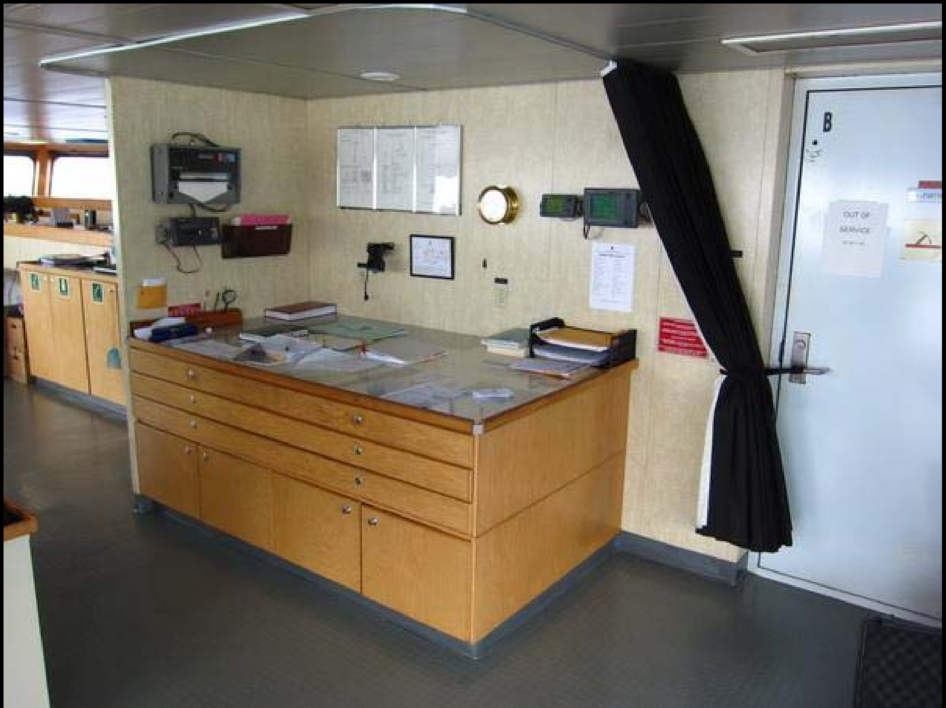
The chart table is located just aft of the forward control station. It has several pieces of dedicated electronic equipment. The door on the right is the elevator. Yes, there is an elevator serving all five of the decks.
