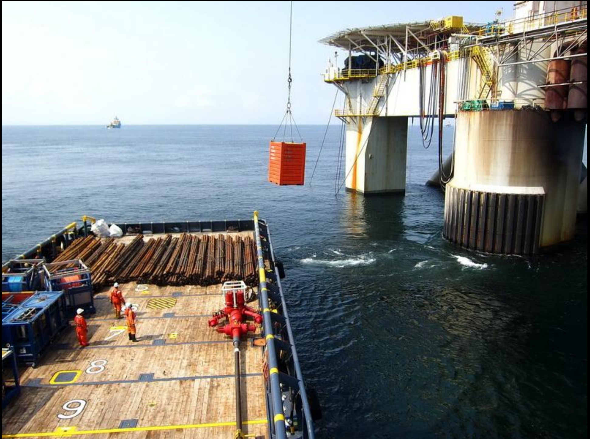
Here you see what the Bourgeois Tide does best, receiving a back load. Notice the prop wash out of the side of the vessel. Dynamic Position computers control the Z-drives, providing a stable position.
