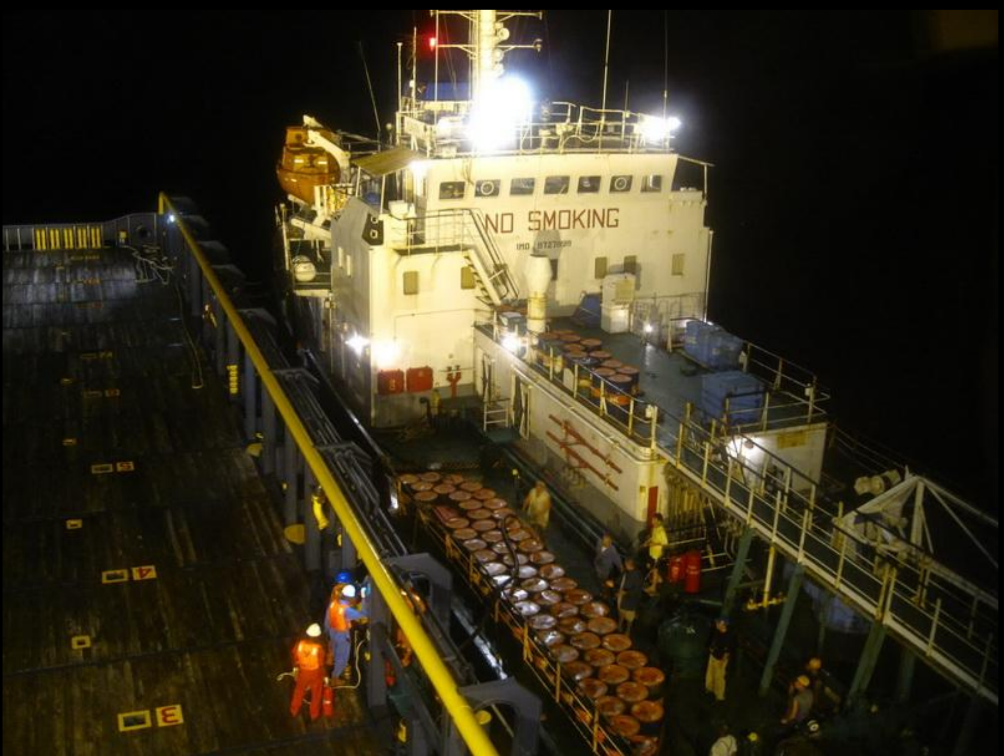
The Gubert Tide is alongside a bunkering tanker offshore Côte D'Ivoire. This is the method for receiving fuel in the area. There must be a very large tax on fuel in Abidjan to justify this kind of operation.
