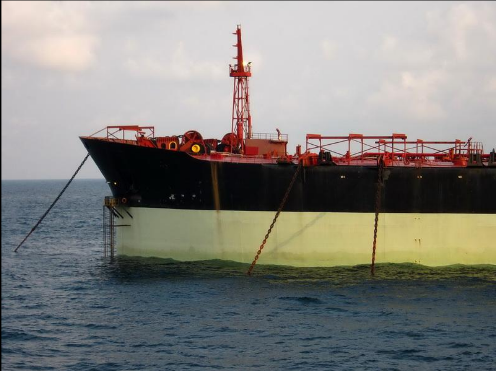
Ten large anchors going off in all direction are used to hold the tanker in one spot.
