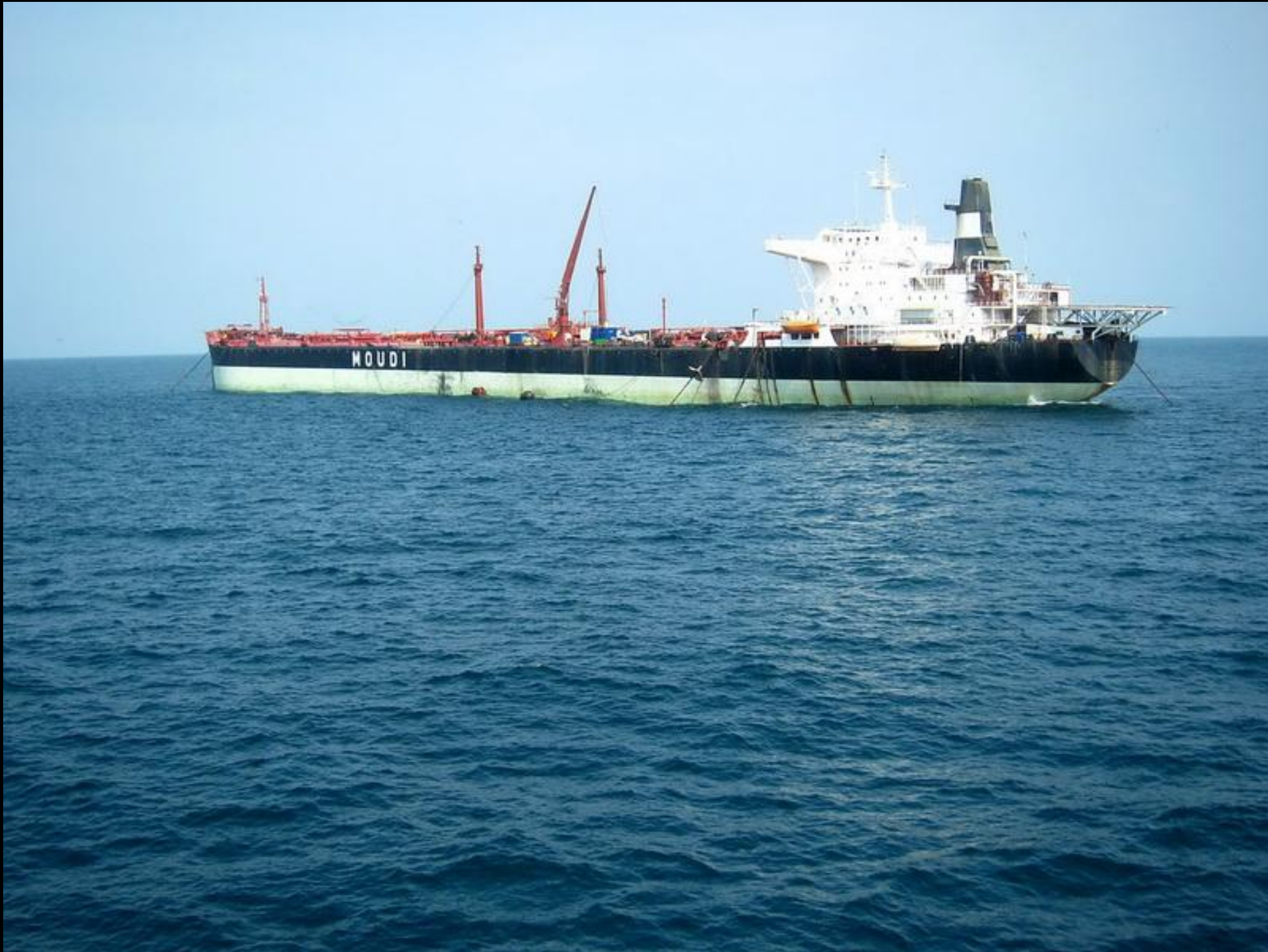
Production flows from multiple platforms and various fields and is stored in this huge tanker for delivery worldwide.
