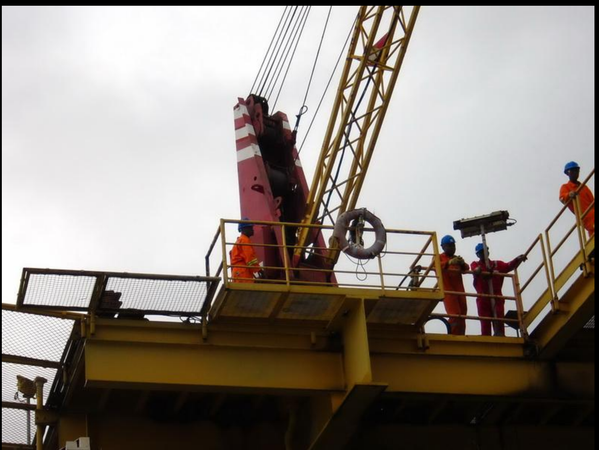
Oddly enough there is no cab for this crane. The operator stands on the deck operating the controls. When the crane slews left or right he has to walk around with the crane to maintain his position on the controls.
