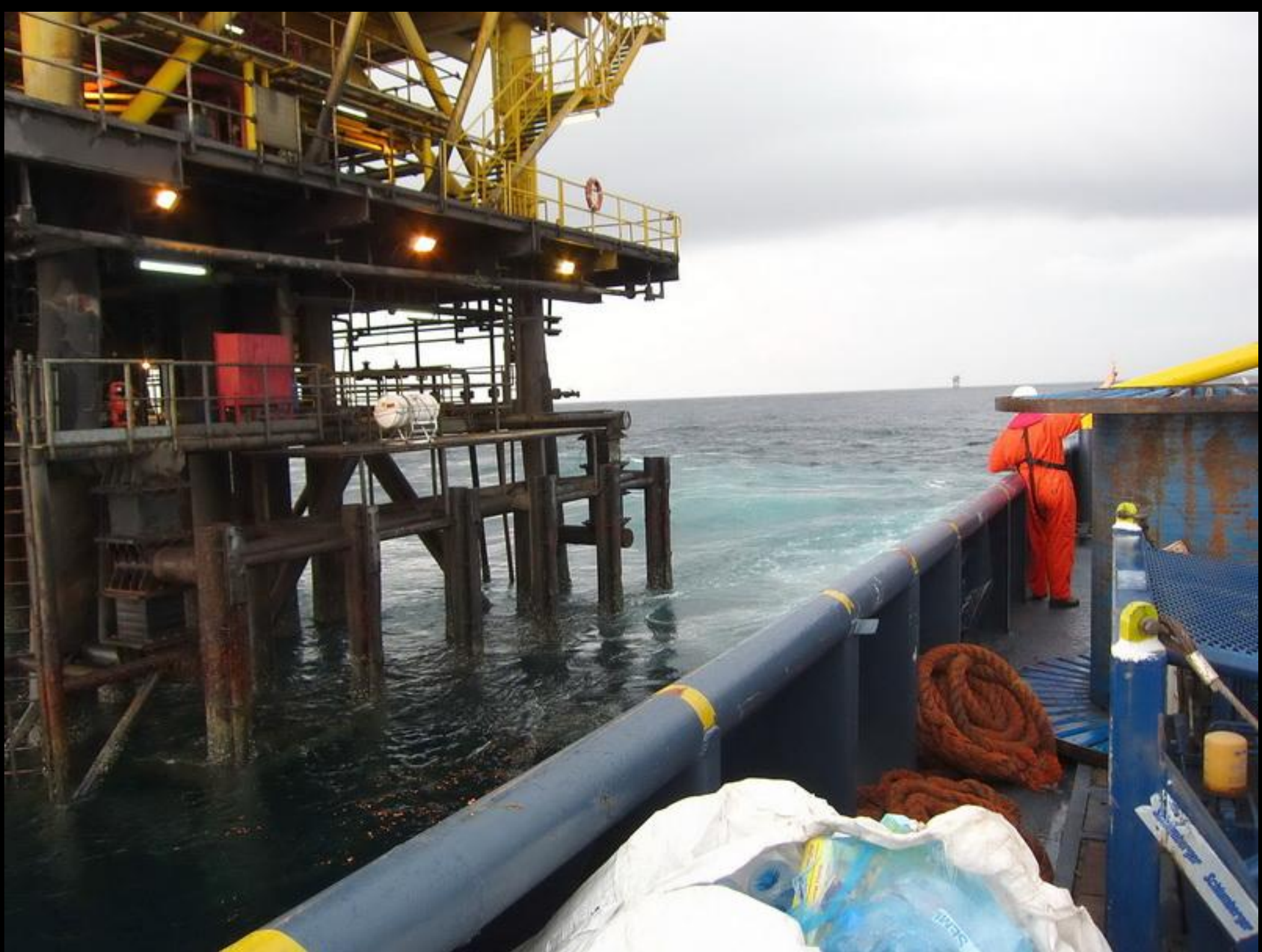
Although it appeared we are touching, five meters is a good standoff distance for a vessel this size not using DP.
